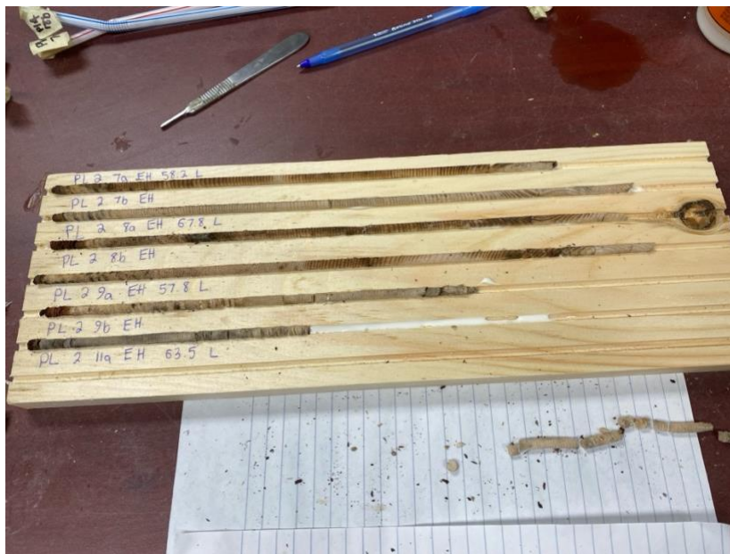
Figure 3.1 Glued and mounted core samples prior to sanding
