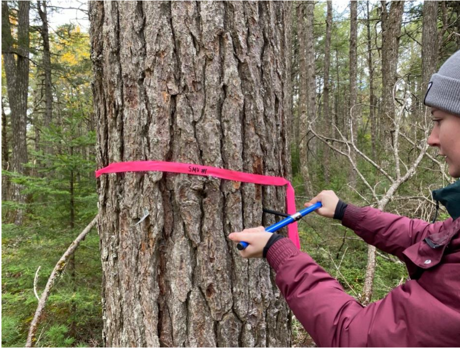
Figure A.1 Sampling with a 5.1mm increment borer
